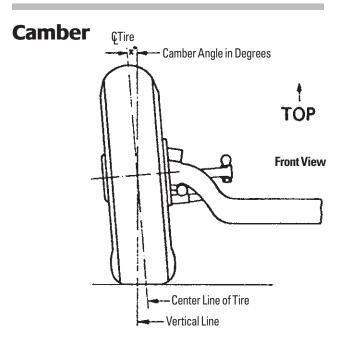
Proper wheel alignment is essential for optimum tire life and vehicle handling characteristics. Alignment settings should be checked with the truck loaded. Alignment adjustments can be made on an unloaded truck: however, modifications in the vehicle manufacturer's alignment recommendations may be required for proper "loaded" settings.
