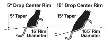
The following diagram shows how the beads of a 16" tire will not seat on a 16.5" rim. The beads should not be forced out against the rim flanges by using more air pressure, because this will break the beads and the tire will explode. Never exceed 40 psi when seating the beads on the rims.
