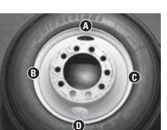
7. Distances A, B, C, and D should be within 2/32". If they are not, break down, re-lubricate and mount again.
