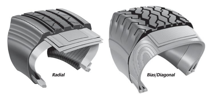
Radial tire body ply cords are placed straight across the tir from bead to bead. In addition, radial tires have belt plies, which run circumferentially around the tires, under the treat They constrict the radial ply cords and stabilize the tread a
