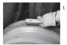
. Remove dirt, rust or corrosion that can interfere with proper seal or damage bead.
