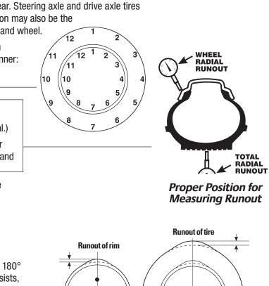
Runout of Tire Due to Runout of Rim
