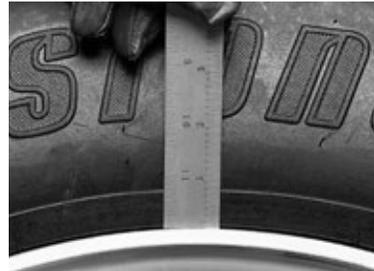
6. Measure distance from molded ring on tire to flange locations, 90 degrees apart.
