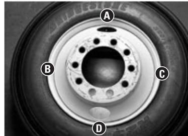
7. Distances A, B, C, and D should be within  $2/32$ ". If they are not, break down, re-lubricate and mount again.
