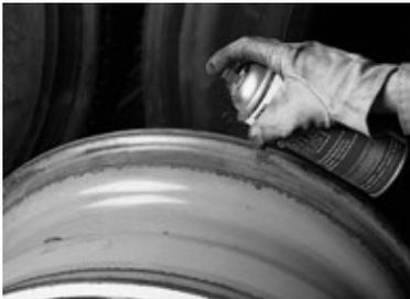
2. Protect bare metal with primer or anti-rust paint to prevent further corrosion. Allow to dry.
