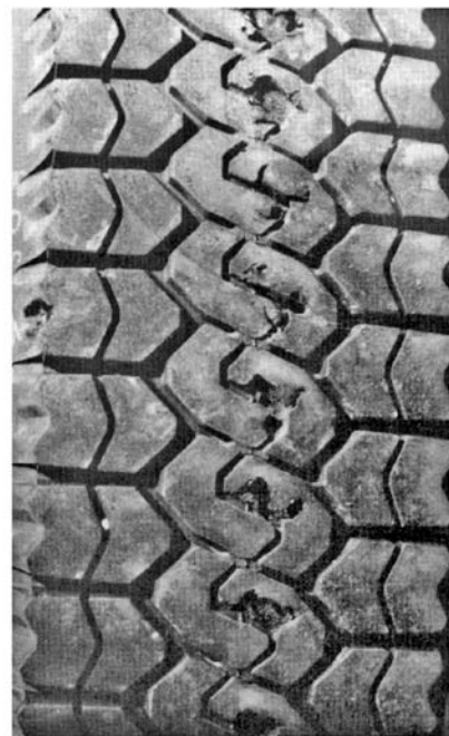
Example of Dyno Damage
