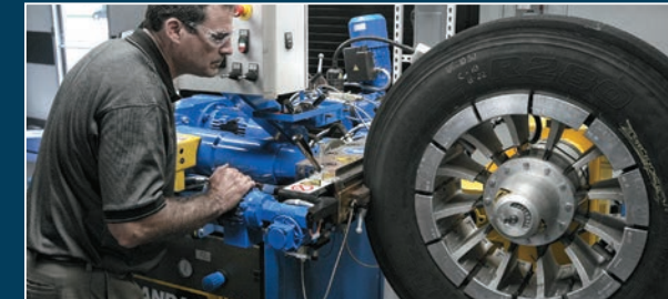
Step 6: Applying Cushion
