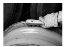
1. Remove dirt, rust or corrosion that can interfere with proper seal or damage bead.
