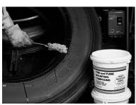
4. Lubricate tire bead. Do not use petroleum or solvent-based products. They cause rubber to deteriorate.
