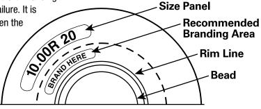
Proper Branding Area on Steel Radial Tire
