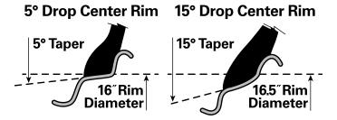
The following diagram shows how the beads of a 16" tire will not seat on a 16.5"rim. The beads should not be forced out against the rim flanges by using more air pressure, because this will break the beads and the tire will explode. Never exceed 40 psi when seating the beads on the rims.
