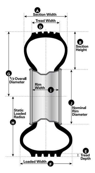
NOTE: Tires mounted and inflated to recommended pressure. All dimensions measured 24-hours after initial inflation.
