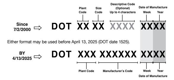
Note that the last portion of the TIN is changed-identifying the tire manufacture date using the same format for week and year. (For tires made before 7/2000, there is one digit for the year.)
