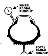
**Proper Position for** Measuring Runout
