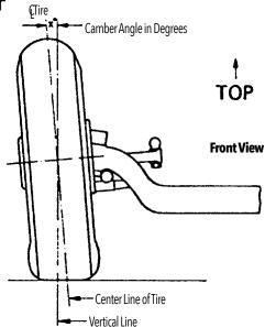
Proper wheel alignment is essential for optimum tire life and vehicle handling characteristics. Alignment settings should be checked with the truck loaded. Alignment adjustments can be made on an unloaded truck; however, modifications in the vehicle manufacturer's alignment recommendations may be required for proper "loaded" settings.
