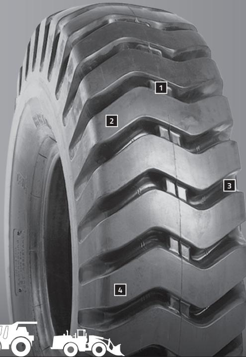
The R-Lug S bias tire is specially designed for reach stackers, top picks, straddle carriers, and other container handling equipment.
