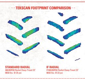
Firestone tires with AD2 technology can carry a given load at a lower pressure than standard equivalent-sized radial tires. Lower pressure gives these tires a larger footprint and helps reduce soil compaction.
