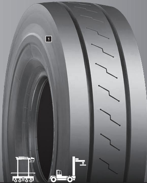
The V-Steel Container Handler-R radial tire is specially designed for reach stackers, top picks, straddle carriers, and other container handling equipment.
